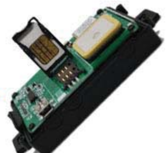
Insert the SIM card and make sure its chips face down
